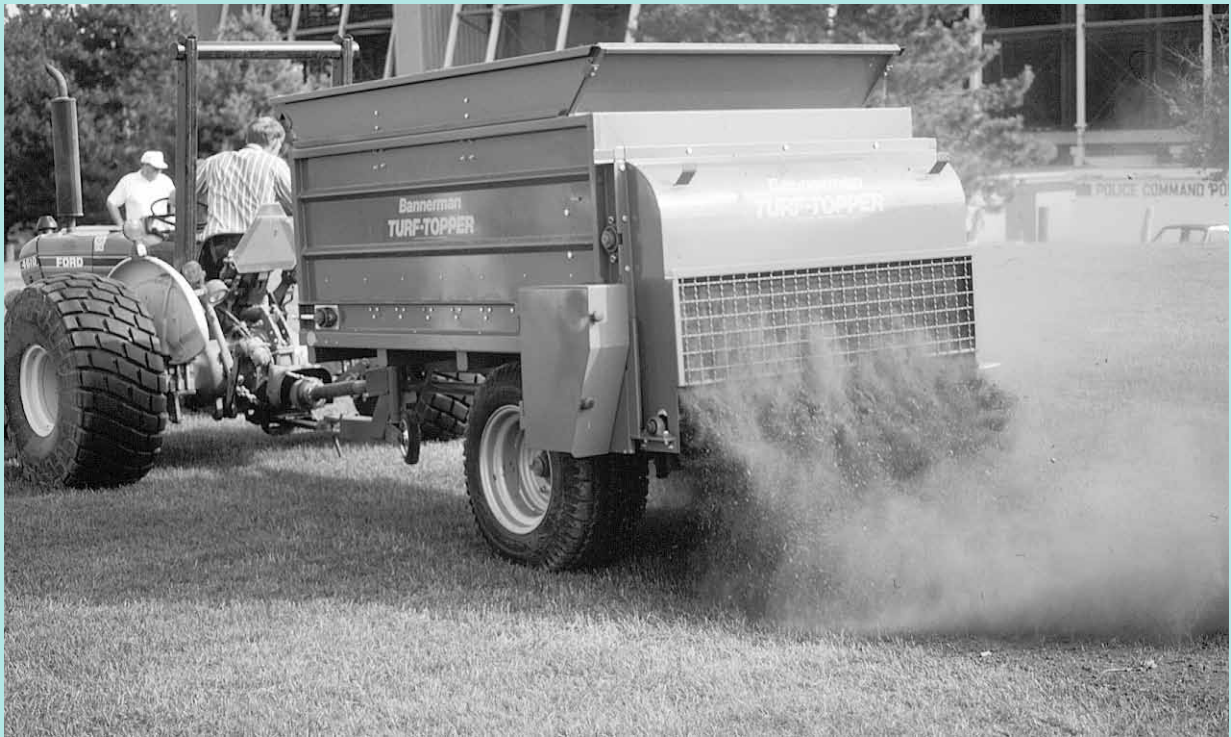
Figure 4. Modified spreaders with conveyor belts and brushes mounted on the back are ideal for surface applications of compost.
